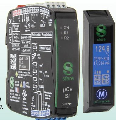
This series has intrinsically safe inputs: they are associated equipment, to be placed in safe area or ATEX/IECEx area 2. They have input circuits for connection to a sensor placed in hazardous area and output circuits for connection only in safe area or ATEX/IECEx area 2.
