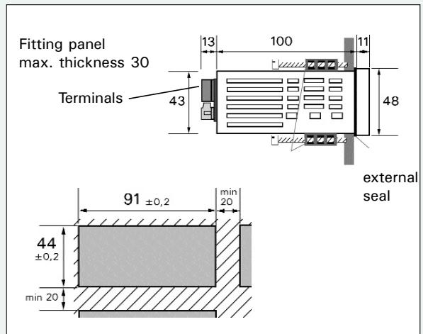
**Mounting:** on panel, cut out 44 x 91 mm
