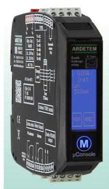
The differential relays ELRv are relays for the limitation of the earth leakage current, of the type A for the ELRv20/30 and the type B for the ELRv21/31. Associated with a measure toroidal and a circuit breaker, they allow to perform on low voltage networks of the type TT, IT, TNS the following functions:
