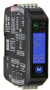
The differential relays ELRv are relays for the limitation of the earth leakage current, of the type A for the ELRv20/30 and the type B for the ELRv21/31. Associated with a measure toroidal and a circuit breaker, they allow to perform on low voltage networks of the type TT, IT, TNS the following functions:
