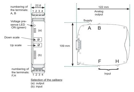
Protection: housing/terminals: IP20 Removable terminal blocks for screwed connections (2.5 mm², flexible or rigid) Weight: 290g (with packaging) Housing: self-extinguishing case of black UL 94VO PA66. Mounting in cabinet: latching on symmetrical DIN rail
